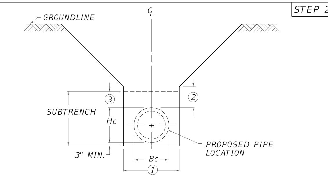
a. TRENCH CONDITION IS WHEN GROUNDLINE ELEVATION IS GREATER THAN Hc ABOVE TOP OF PROPOSED PIPE.
